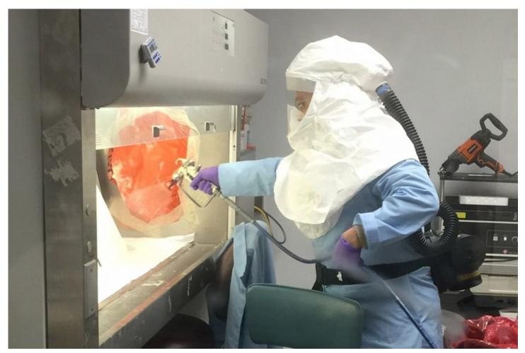
A CCDC Chemical Biological Center researcher sprays Bioxy on contaminated panels to test its effectiveness. Photo credit: Jack Bunja |
